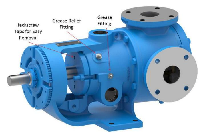
Viking's Chocolate Series pumps offer a number of other standard features to ensure reliability, including jacketing on the head and bracket to melt chocolate before startup; drilled idler gear with hardened iron bushings to prevent caramelization; hardened steel shafts; and steel or ductile iron rotors for high viscosity. All materials are food grade, and the pumps are marked as EC-1935 compliant to prevent leaching of harmful materials into food.
