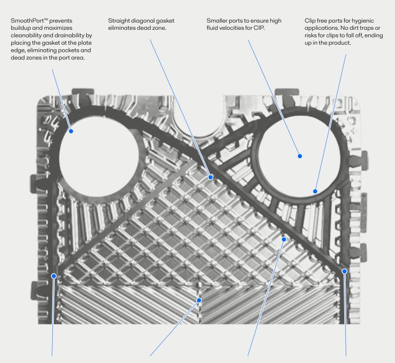
Hygienic gaskets with single ridge secure sealing and superior hygiene simultaneously. CleanChannel<sup>™</sup> in the HTA and along the gasket makes draining easier during cleaning and facilitates the flushing of remaining particles, such as flakes of fouling and fibers. Beam knobs with rounded design avoiding dead zones and allowing cleaning fluids to access all surfaces. Hygienic leakage groove ensures that any leaking fluid from the diagonal or port gasket is detected without delay.
