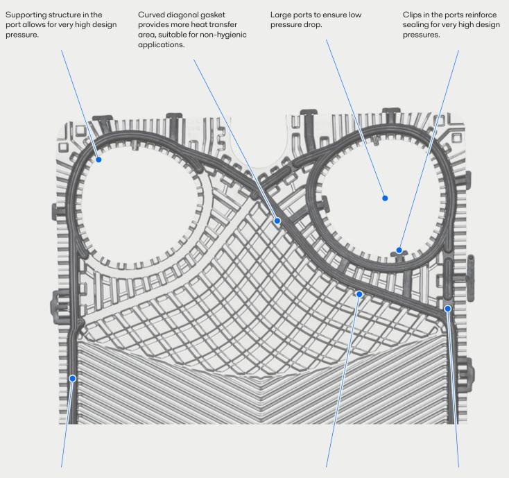
Industrial gaskets with three ridges distributing gasket forces to secure maximum sealing also at very high operating pressures. Square beam knobs in robust design for very high design pressure.
